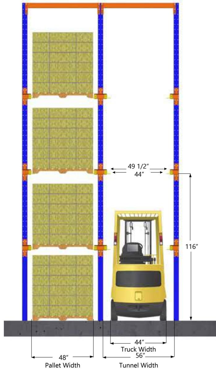
Many palletized loads are transported by road or rail stacked 2 high. This characteristic is often utilized in Drive-In systems for the floor location, to gain valuable vertical space.
